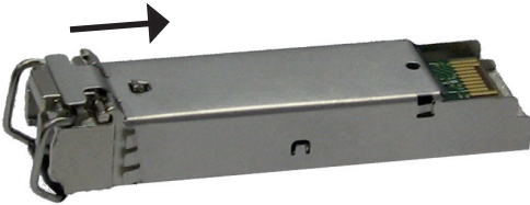
Figure 26: F/O SFP transceiver
